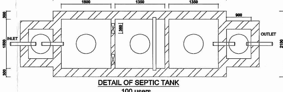
DETAIL OF SEPTIC TANK 100 usrs
